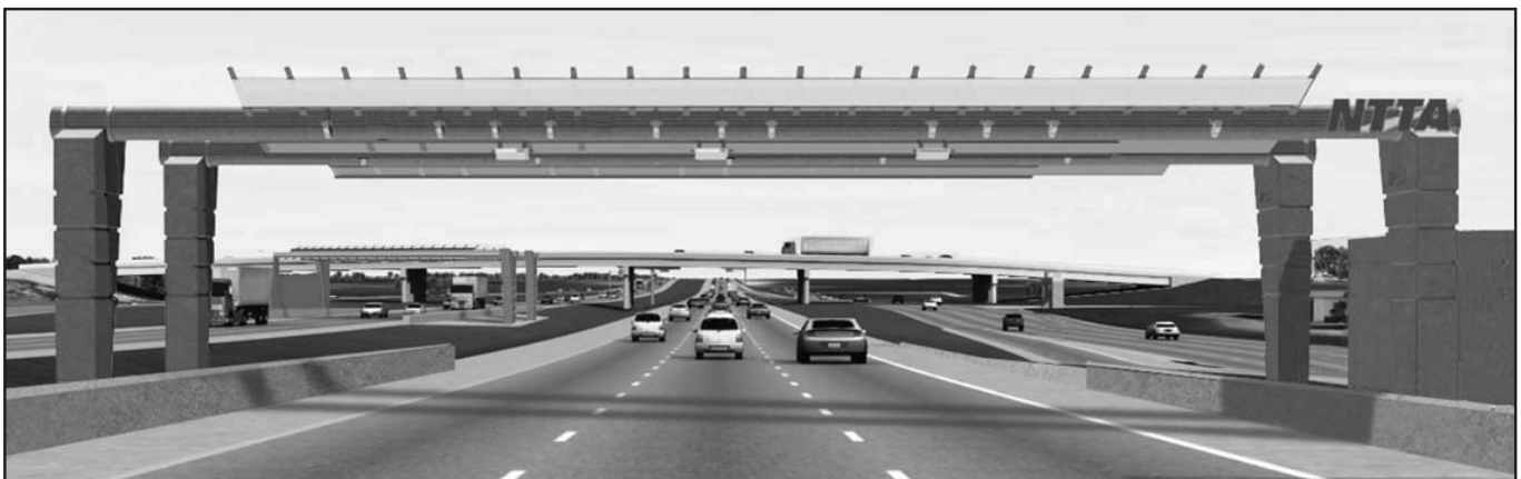
Figure 2 – Main lane ETC gantry 3D view
